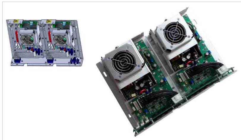
Figure 1: CAD drawing & photo of completed semi-custom design for a high-rel radar implementation within a space constrained enclosure
