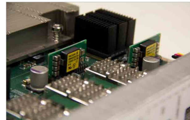
Figure 2: A digital POL regulator in single in-line packaging saving board space and improving cooling
