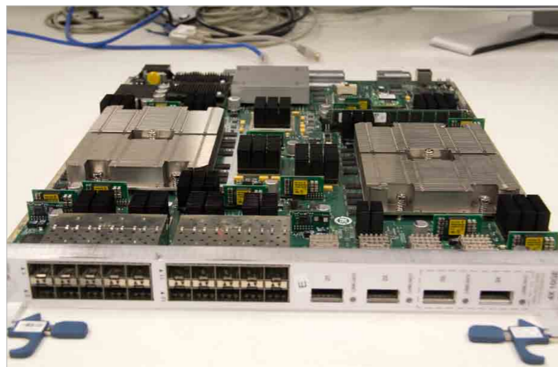
Figure 1: Ericsson's high-end subscriber management and routing board from passive 'Board Mounted Power Sources' (BMPS) that only supply power to loads, to very advanced combinations of hardware and software that make a contribution towards the full integration of board power within the digital chain. Pushing the limits The challenge for the board power system designer is to predict what will be required in terms of increasing power, decreasing board-space, higher flexibility and lower power consumption by the final end-application network data processor. Leading-edge equipment designed to handle high levels of data traffic is often based on multiple cores or processors that are not always fully available at the time of system development. And this equipment requires highly sophisticated power management with power sequencing, monitoring and the capability to dynamically modify an element of the power scheme to adjust to traffic conditions and thereby enable a reduction in energy consumption. An example of this type of complex equipment – an Ericsson high-end subscriber management and routing board – is shown in Figure 1 .
