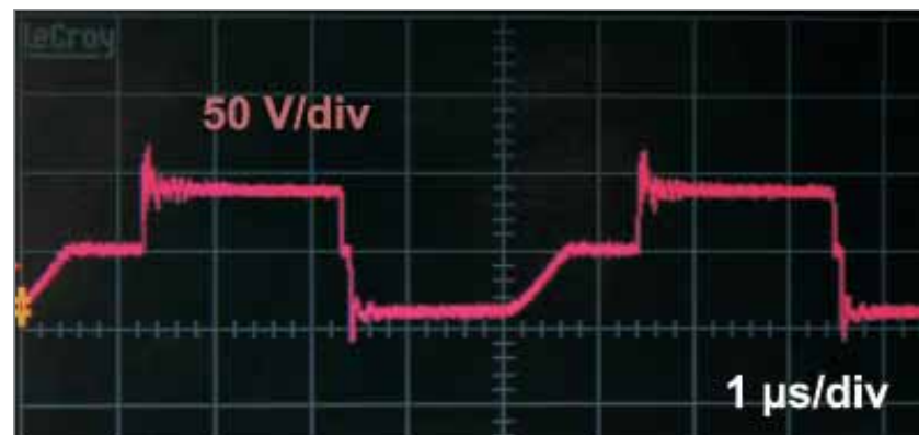
Figure 2: Secondary forward diode voltage waveform, VD, with 100 VAC applied and no snubber
