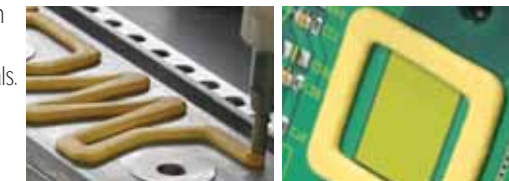
Gap Filler 1500 has natural tack and cleanly flows into position for final assembly without leaving thermal material behind.
