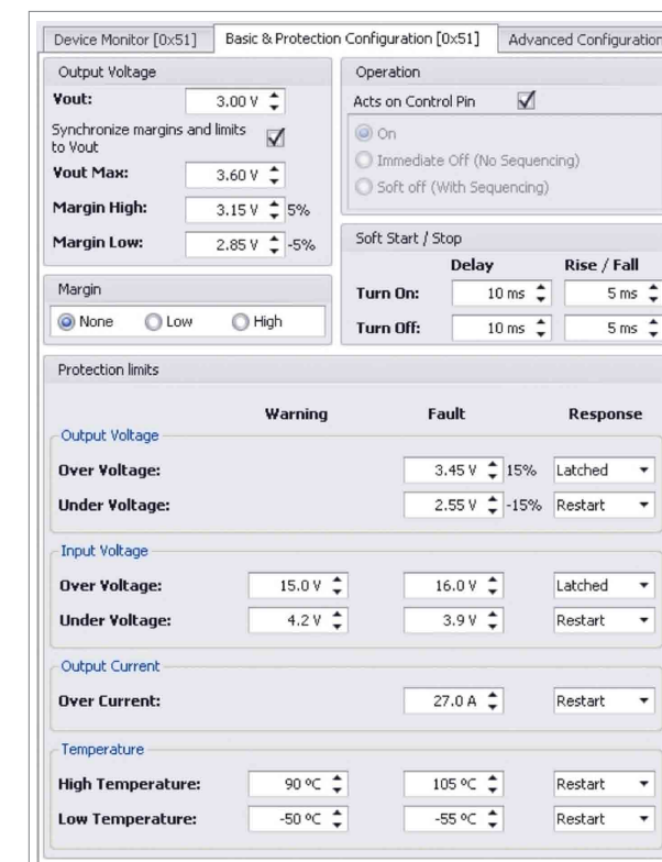
Figure 3: A GUI simplifies PMBus-device set-up tasks.
