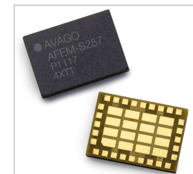
Figure 2: Amplifiers, switches, and filters are all encapsulated in a single package for simple layout
