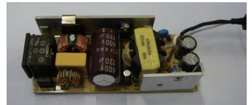
Figure 1: 65W demo board of the TEA1733 Fixed frequency flyback converter
