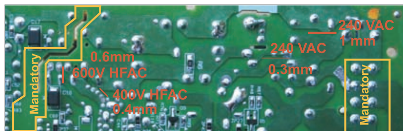
Figure 3: Example Preproduction Power Supply Board with Inadequate Spacing.
