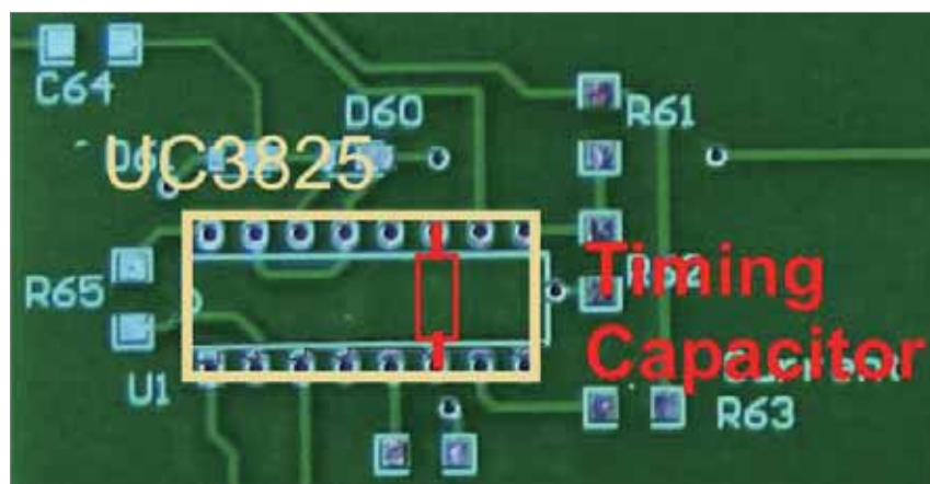
Figure 2: Detail of Control Chip
