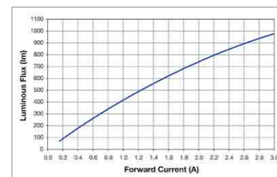
Figure 3: Cree XM-L Luminous Flux vs. Current (25°C)
