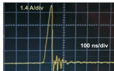
Figure 5: Current sense waveform with high-line voltage input and short-circuit on output. Notice that the current pulse is reduced to just 100 ns. When this current signal exceeds a second current limit threshold, soft-start is reinitiated, and the converter enters a burst mode of operation at low frequency, protecting the semiconductors from overstress.
