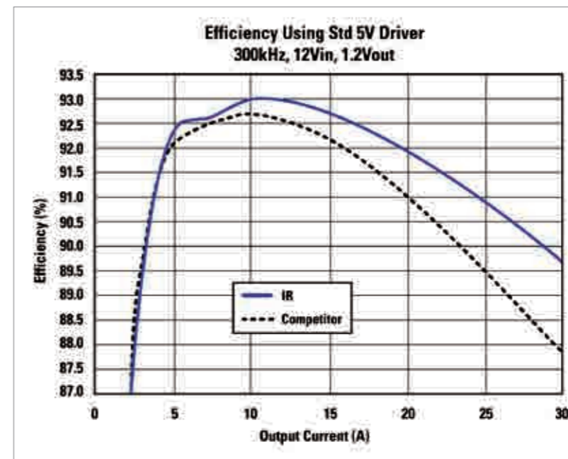
Figure 3: Efficiency improvement by reducing MOSFET R_g .
