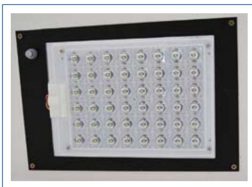
Figure 4: Designers can select the Dolphin light source, Phoenix, for their own lighting fixture housing design.
