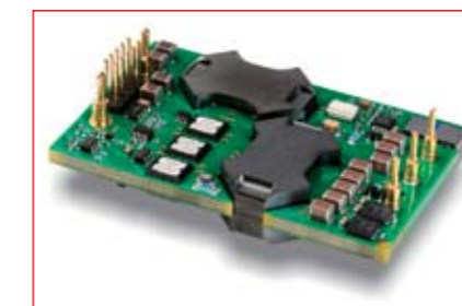
Figure 5: Innovative through-board mounting helps facilitate the converter's quarter-brick format.
