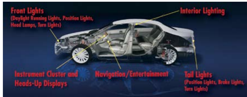
Figure 1: HBLEDs are making inroads into every lighting application in a car - from headlamps to brakelights and everything in between.
