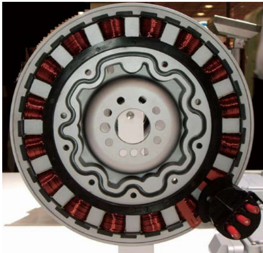
External Rotor, as used in SUVs by BMW, made by ZF Sachs AG (Formerly knows as Fichtel & Sachs and later Mannesmann Sachs).
