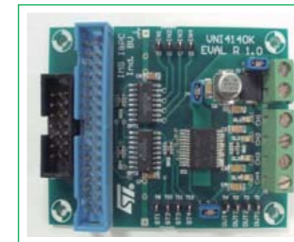
Figure6: VNI4140K reference demo board.
