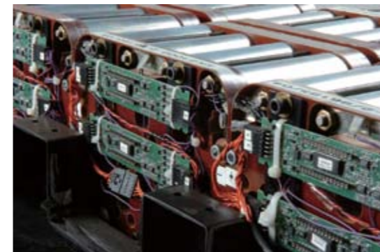
A row of plug-in hybrid electric vehicle (PHEV) battery cells (Photo courtesy of Argonne National Laboratory).
