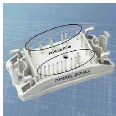
Figure 2: Power Line and Control Pins reside on opposite sides of the package
