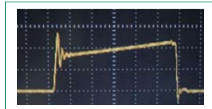
Figure 5: Current waveform for well-behaved converter.
