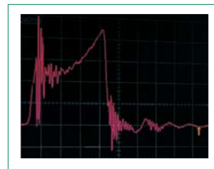
Figure 7: Current waveform with transformer saturation during startup.
