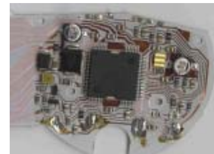
Figure 5. PC-board of mechatronic mirror. Smart power chip is in center position.
