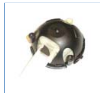
Figure 6. Housing shell for motors and PC-board
